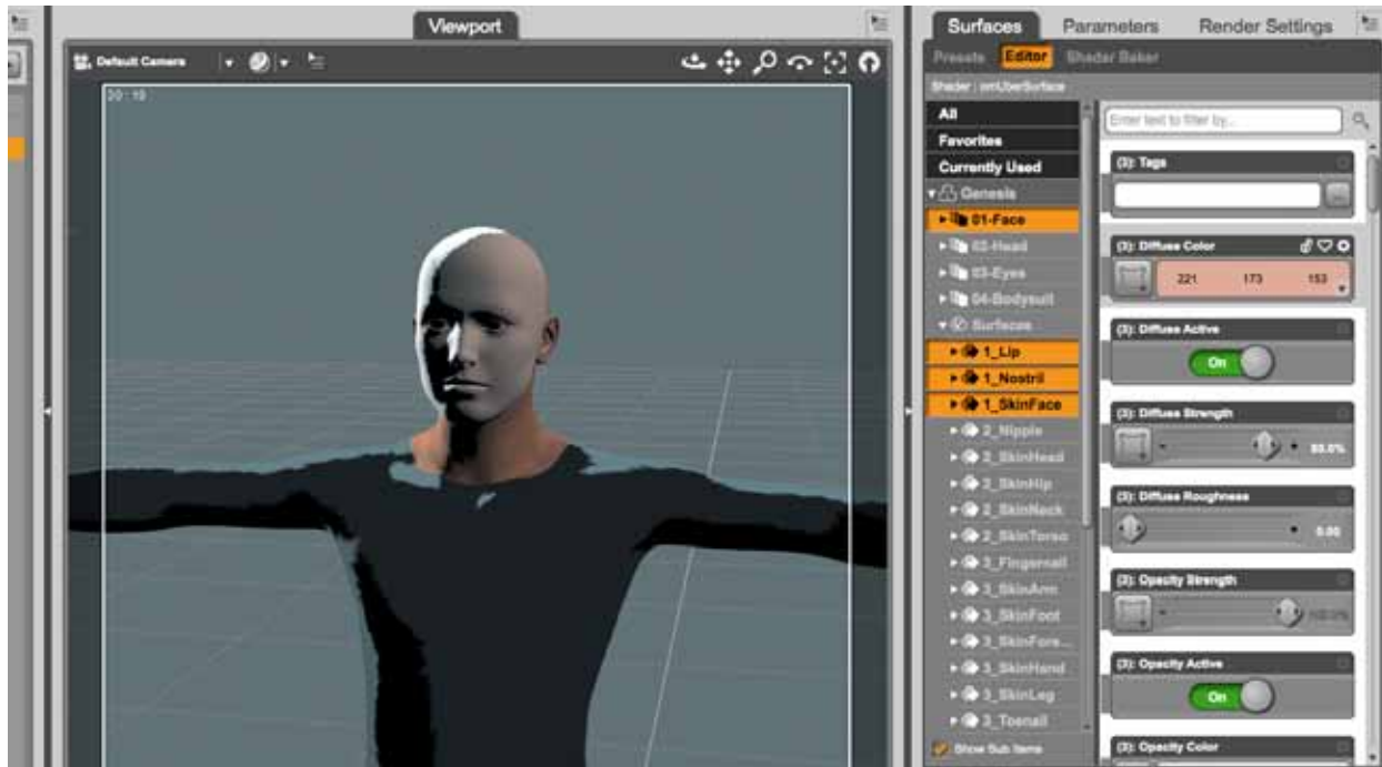
Figure 17: Face texture removed. It appears a bit blue because of the specular color.
